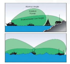
Shakespeare combines a normal beam width with a unique low angle of radiation to minimise signal fading in rough or rolling seas.
