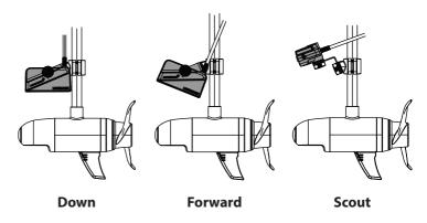
The transducer can be mounted on the port or starboard side of the shaft.
