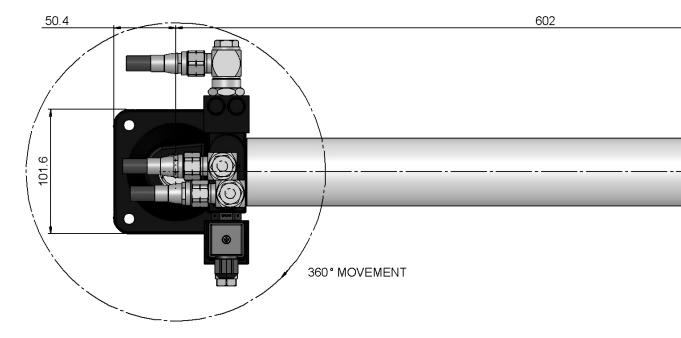
Ensure that cylinder rod movement is limited by the Steering end-stops and not by the actuator.
