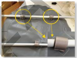
Longer Velcro patches, which will roll all around the rail for greater bonding strength.
