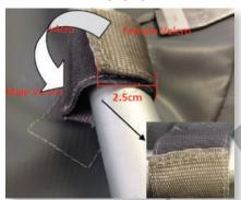
1. Only 2,5cm (length) female Velcro used for bonding.
